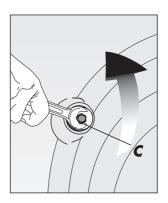
"C", should be turned in a anti clockwise direction until the bolt can be partially withdrawn.
